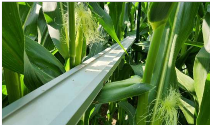
Figure 3. Swathing system erected at ear-height inside a corn canopy to re-evaluate ESW.
