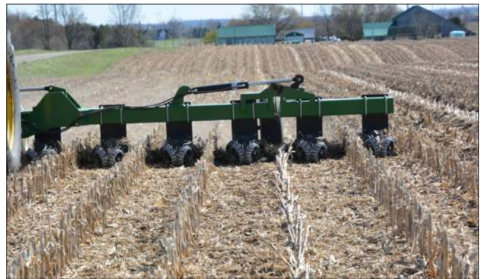
Figure 2. A row cleaner clearing corn residue in the area to be planted.
